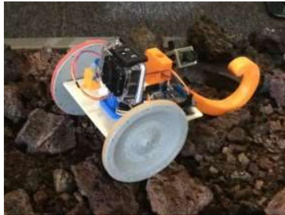
Figure 8 – 3D printed rover
