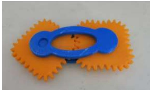
Figure 12 – 3D printed square gears
