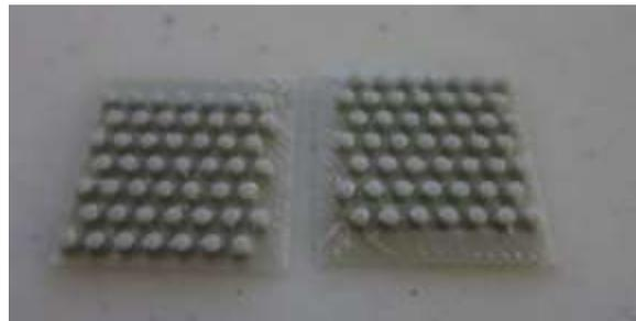
Figure 13 – 3D printed velcro alternative
