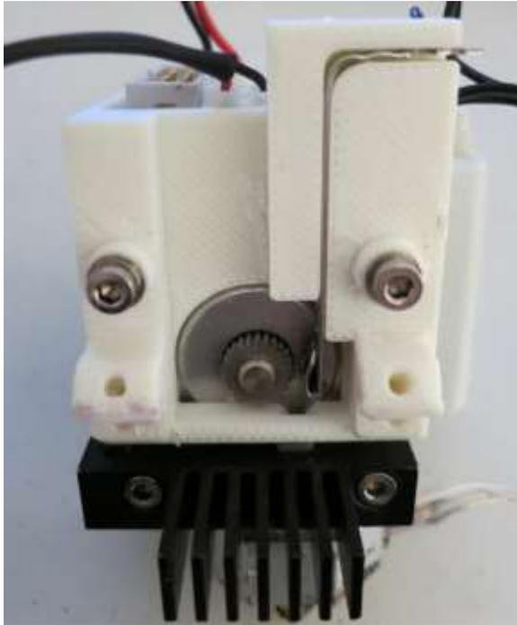
Figure 9 – Replacement extruder mechanism
